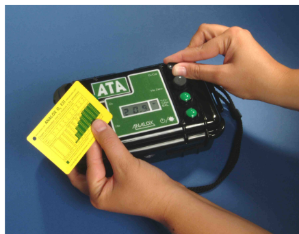
O 2 calibration in clean air
